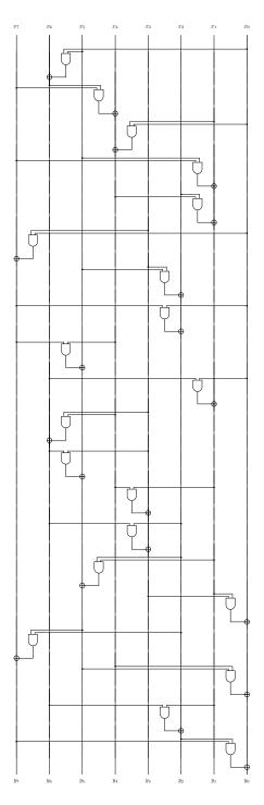
Fig. 4. A 40-gate TI-friendly circuit of the 7-8-64 S-box of Table 3
