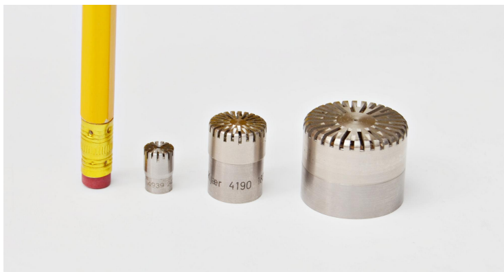
Figure 2: Microphone capsules (from right to left): Brüel&Kjær 4145 (1" diameter), 4190 (1/2" diameter) and 4939 (1/4" diameter). A common pencil is included for size comparison.
