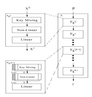
Fig. 1. Structure of an R-round block cipher E
